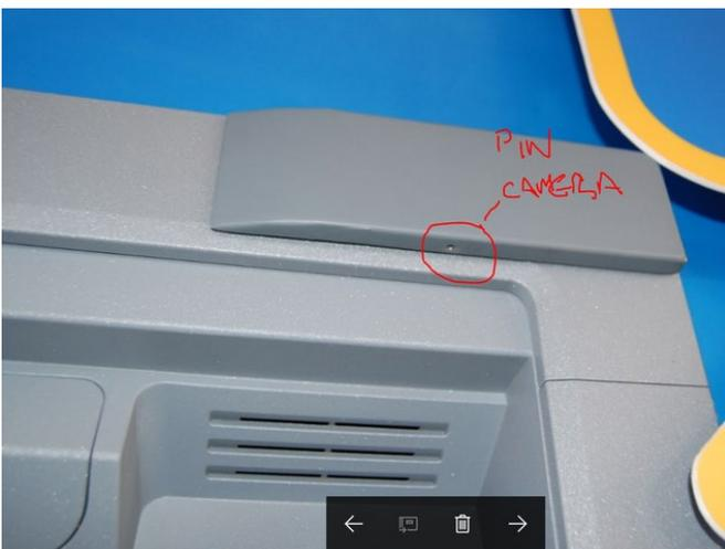
**Pin Camera** – This is an example of a camera that could be attached to a through-the-wall, walk-up or drive-up unit. There is a color difference in this example, and it is bumped out from the actual machine fascia. To a member using the machine for a withdrawal, something like this is likely to be overlooked unless they are more familiar with the aesthetics of a machine.
