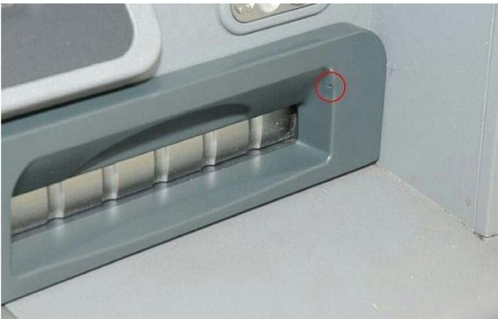
This is an example of a camera overlay on the cash dispenser area. The color of the attachment does not match the fascia however it probably matches the factory dispenser cover and the depositor cover.
