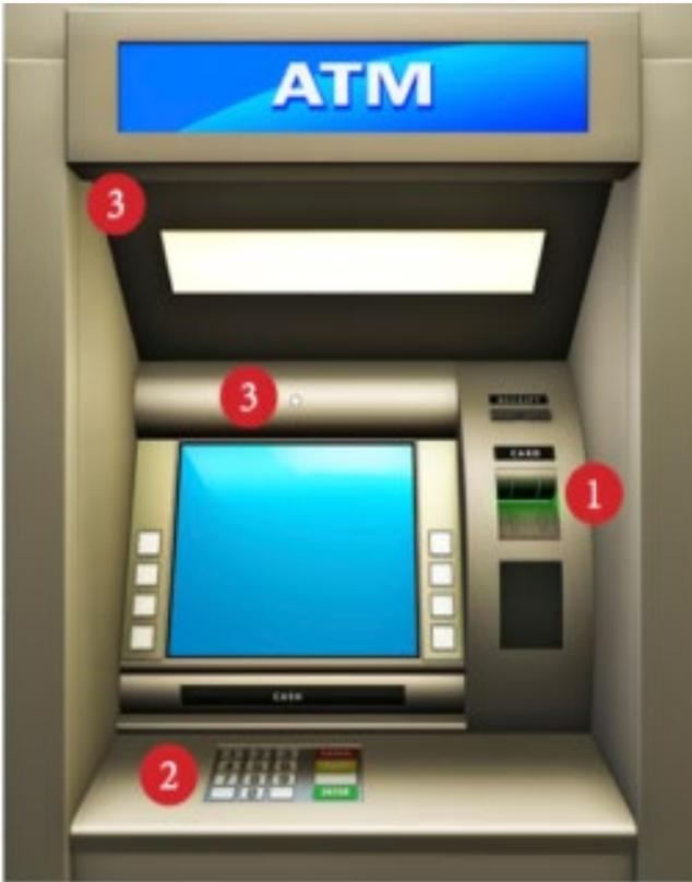
1. **Card Reader** – Overlay card skimmers/readers can be placed and removed quite quickly and easily, check your card readers daily by pulling gently. On the contrary, deep insert card readers are not detectable by the eye because they are completely inserted into the card reader.
