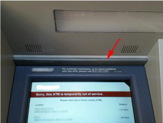
This is an example of a bar camera that is placed right above the screen. Notice that there is a color difference compared to other parts of this ATM, however, the screen frame and unit color is not the same either. The arrow is pointing to the small camera eye.
