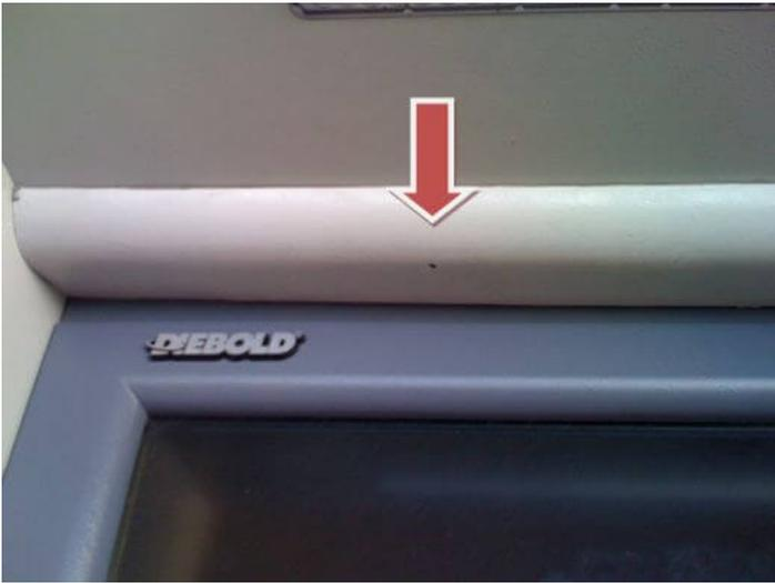
We do not have Diebold units, but notice this is rounded compared to the bar example before. This example is much more of a color match than the previous examples as well. Take notice again of the small hole, which is the camera eye that collects member's PINs during their transaction.
